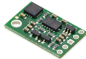
Figure 2.6: A Pololu MinIMU-9 v2 IMU. Taken from [27].
