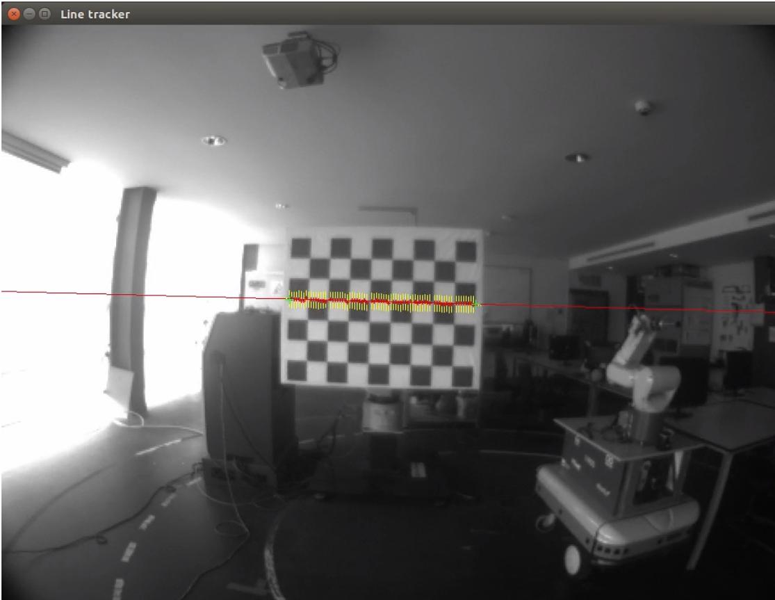
Figure 3.6: Results of the ViSP line tracking method.
