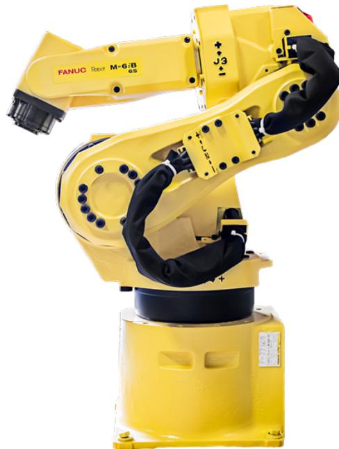
Figure 2.7: A FANUC M-6iB/6S robotic manipulator. Taken from [31].
